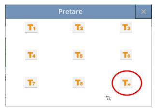
2. Press the **T**<sub>+</sub> key, circled above, and a numeric entry screen, shown below, appears.
